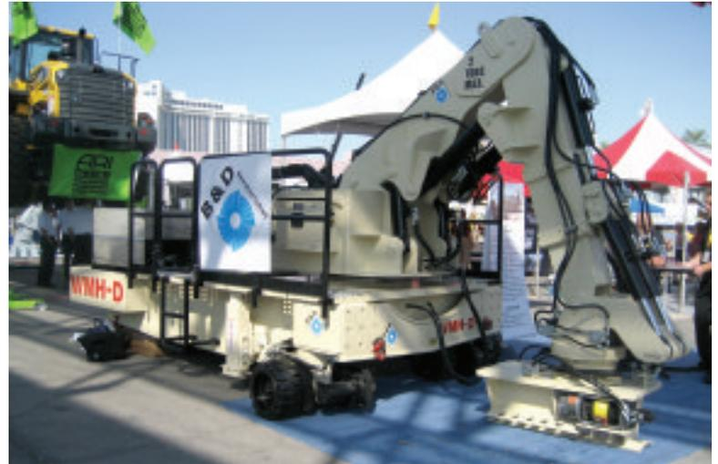
B&D Manufacturing's WMH-D Multi-Handler is a remote-controlled machine that can remove and replace wheels, motors, struts, cylinders and spindle brakes.
