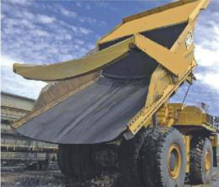
*Duratray SDB pf 172 m capacity with tailgate mounted on SDB Komatsu 830E*
